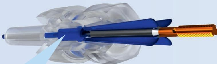
Internal coolant supply (max 50 bar) for optimum supply of lubricant through the collet chuck slots directly to the cutting edge of the Tapping.
